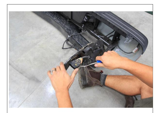
8. Remove the trailer wiring harness, by releasing all the clips securing it to the factory bar with a trim tool. Set aside for refitment to Offroad Animal bar.
