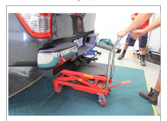
1. Before beginning work, support the factory rear bar / tow bar using lift trolley or jack.
