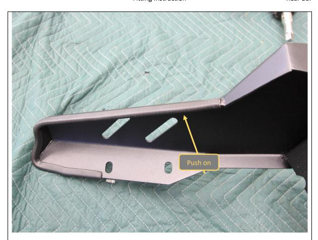
30. Fit rubber pinch weld to lower edges of wing, in the location shown by pushing rubber over the edge.
