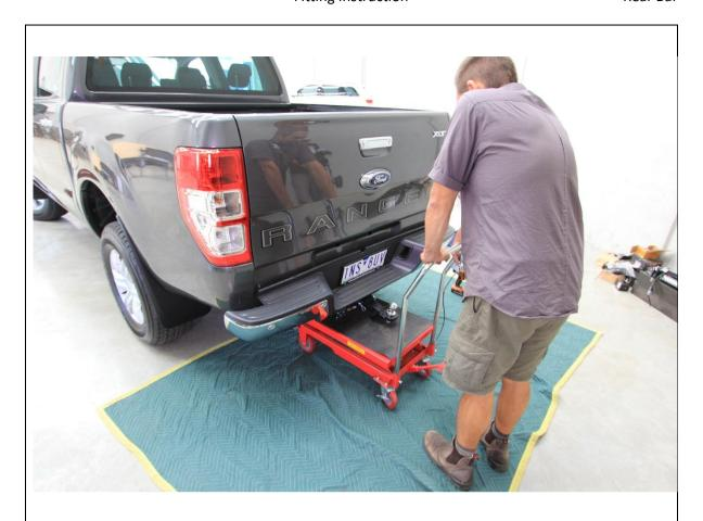
7. With all fasteners removed and the factory bar/ bumper assembly free, carefully lower, then remove from vehicle towards the back once clear of the lower tub panels.
